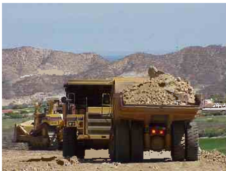
Euclid 769: large-capacity dumper for bulk earthworks
